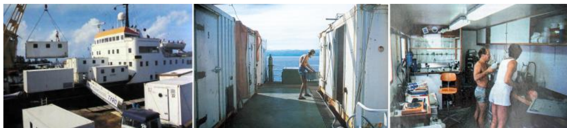
Figure 4. RV Tyro was a unique and fully containerized research vessel. View of the container deck and inside a research container. © SOZ/Fred Hoogervorst.
