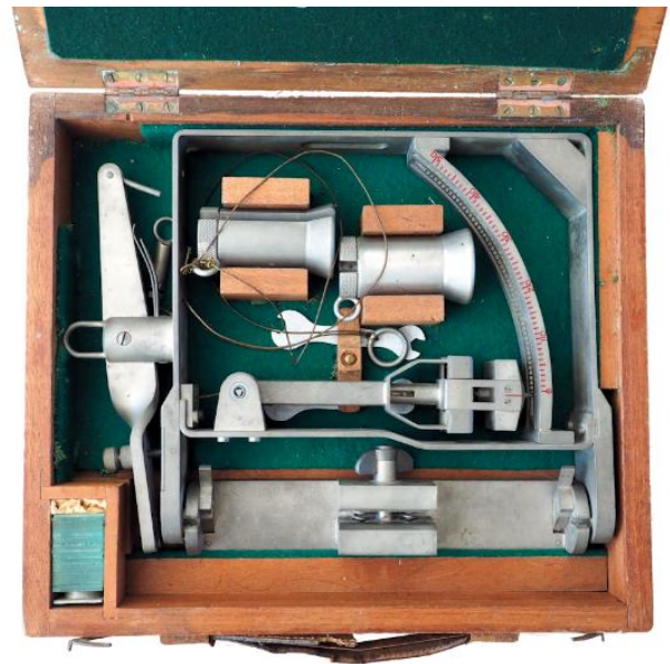
Figure 2. Carruthers and Woods Wire-Angle Gauge with two messengers in its original box (Photo: Clive Holden)
