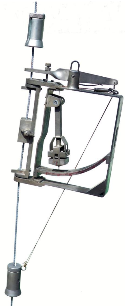
Figure 1. Carruthers and Woods Wire-Angle Gauge suspended on a hydrowire (Photo: Clive Holden)
