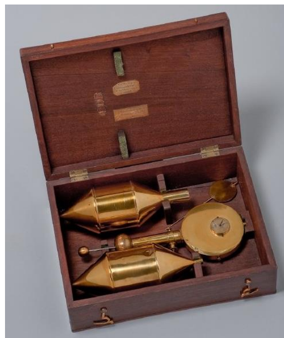
Figure 5. The scale model of a Bathometer at the Museum of the American Philosophical Society in Philadelphia (Cat.Nr. 58.51)
